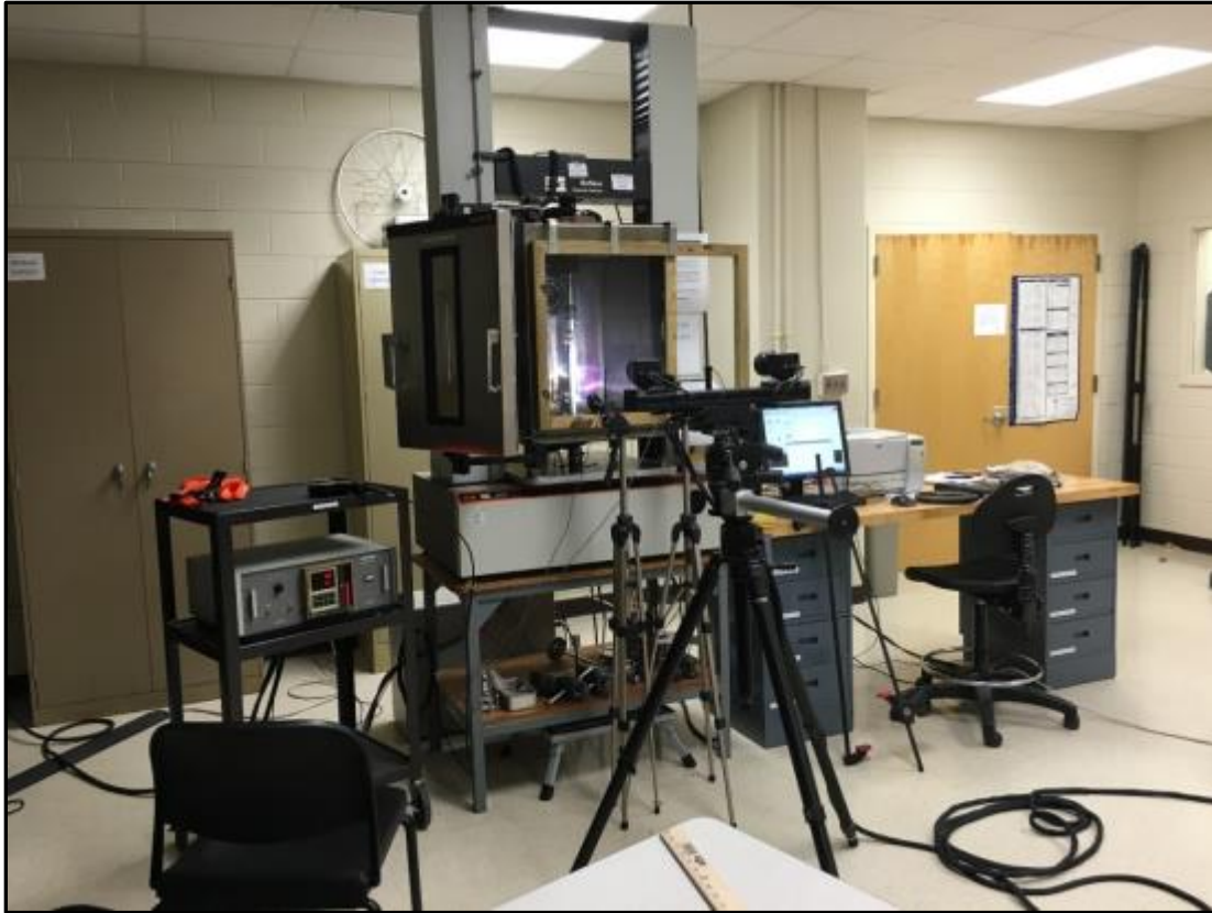
Figure 2-4. Screw-driven Instron frame with 50 kN load cell and oven when DIC measurements were done
