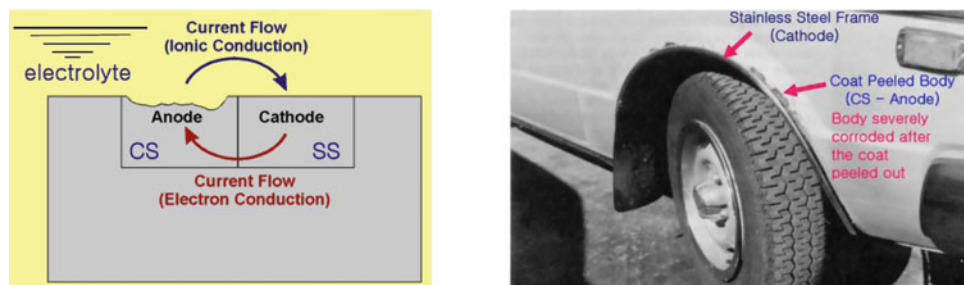
Figure 2.77 Galvanic corrosion on CS in the contact of SS and CS in corrosive environment. (Source: ASM Metal H/B vol.13)
