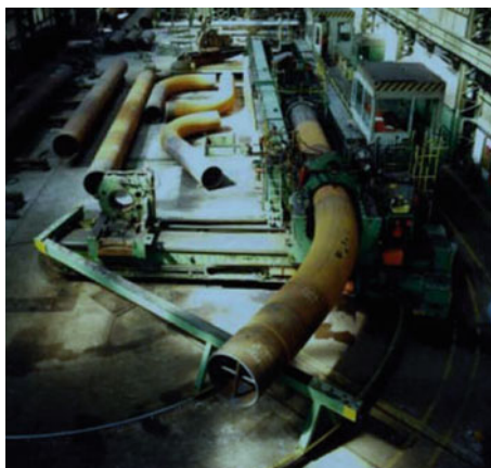
Figure 3.9 Hot Induction Bending of NPS 48 Pipe. (Source: Mannemmann Paper for Oil and Gas Industry International Symposium, 2006Mannemmann brochure, 2013)
