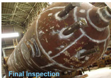
Figure 5.1 Vessel for final inspection
