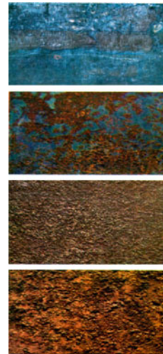
Figure 2.144 Rust grades. (Source: ISO 8501)
