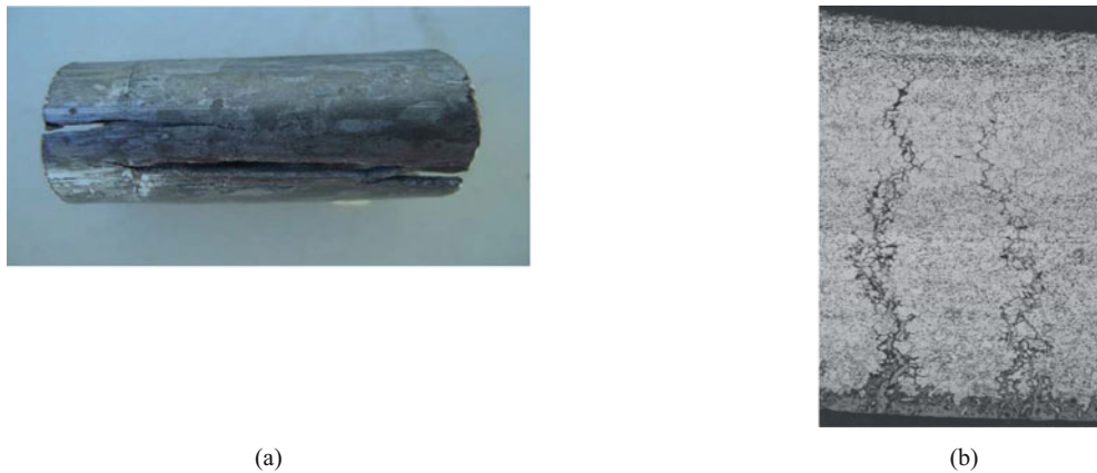
Figure 2.92 Failure of Cupronickel (90Cu-10Ni) tube in wet H 2 S service. (a) Cracked cupronickel (90:10) tube in wet H 2 S service. (b) IGC of Cupronickel (90:10) tube
