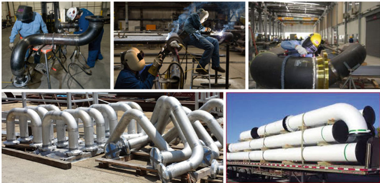
Figure 3.8 Fabrications of piping spools
