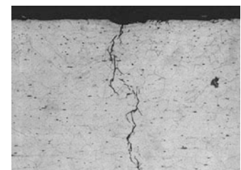
Figure 2.71 Caustic SCC of 304 SS
