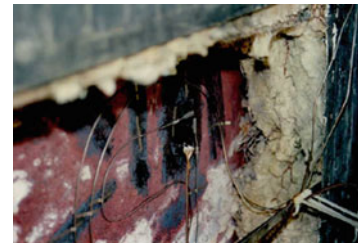
Figure 5.31 Hoop and axial strain gauge installed on a coke drum
