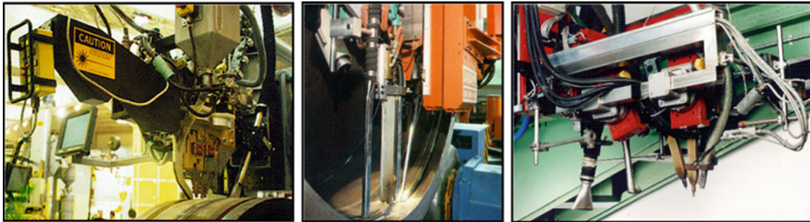
Figure 4.9 Several welding machines for tandem SAW (an example)
