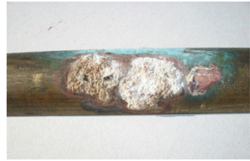
Figure 2.95 Dezincification corrosion of brass
