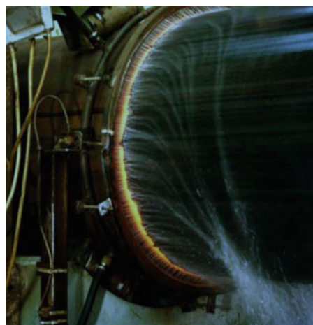
Figure 3.10 View on Induction Coil and Heated Zone During Bending. (Source: Mannemmann Paper for Oil and Gas Industry International Symposium, 2006Mannemmann brochure, 2013)
