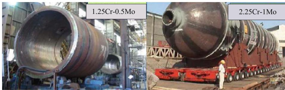
Figure 2.12 Cr-Mo steel reactors with 150–300 mm (6–12 in.) thickness. (Source: Doosan and JSW brochures, 2005)
