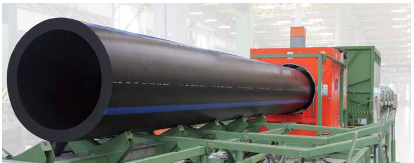
PE 100 Ø 1200 mm PN 16 pipe wall thickness, s:109.1 mm
