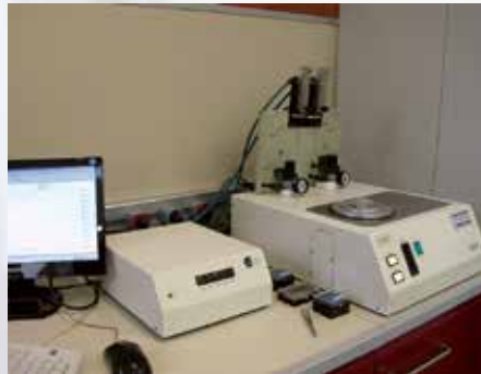
Oxygen Induction Time Test
