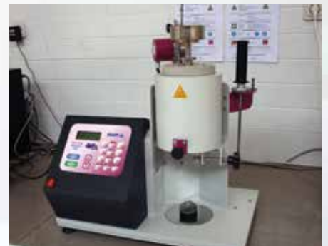
Melting Flow Rate (MFR) Test
