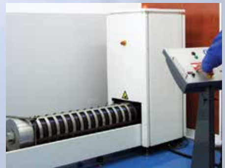
Rapid Crack Propagation Test
