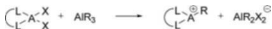
Scheme 2.1 Catalyst–cocatalyst reaction to form an active site having a coordination vacancy. The transition metal center is represented as A, ligands as L (for instance, cyclopentadienyl rings for metallocenes), X are halogen atoms (usually Cl) and R is an alkyl group.
